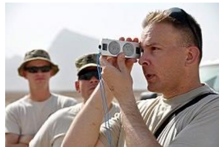
U.S. Air Force Maj. Ryan Schenk, foreground, with Air Mobility Command assigned to the Army's 4th Brigade Combat Team, 10th Mountain Division, demonstrates to Service members with the Farah Provincial Reconstruction Team (PRT) how use a clinometer to measure glide slope obstructions near the Farah, Afghanistan, aircraft landing zone July 30, 2013, during landing zone safety officer training. Farah PRT's mission was to train, advise and assist Afghan government leaders at the municipal, district and provincial levels in Farah province.
