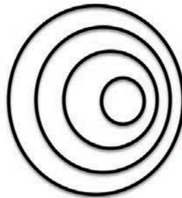
Figure IB. Emission of waves from source moving to the right.
